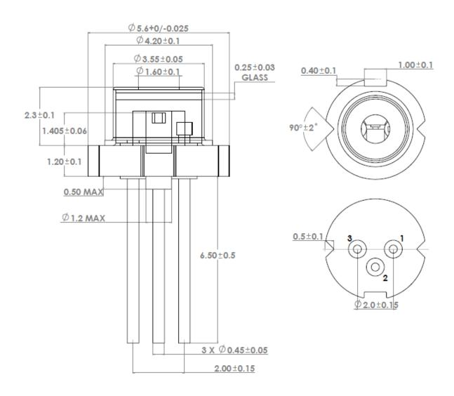
Note : Tolerance is  $\pm 0.05 \text{mm}$  for items without tolerance marking
