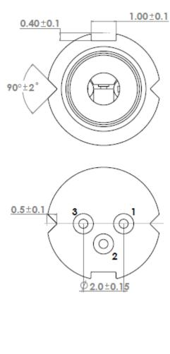
Note: Tolerance is  $\pm 0.05 \text{mm}$  for items without tolerance marking
